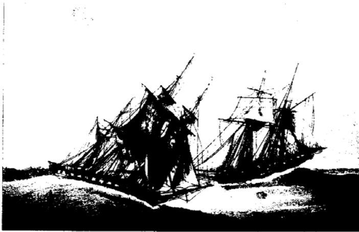
Fig. 1. Two ships roll heavily on a long swell and there is no more wind to damp their rolling. In this situation a strange force, "une certaine force attractive," will pull the two ships toward each other. From P. C. Caussee: "the Mariners Album," early 19th century.
